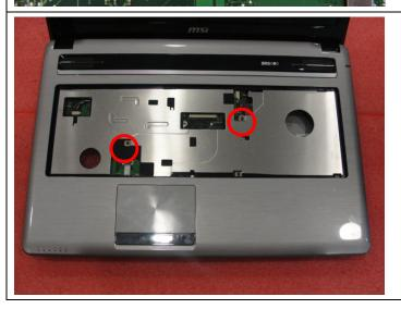
6.8: Remove the 2 screws (M2.5\*4mm). then remove the upper case.
