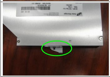
5.3: Remove 2pcs (M2\*3mm) Screws; Then remove ODD Bracket as below.
