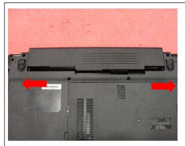
1.1: Move the "Unlock' button base on left picture shows.
