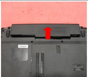
1.2: Release the "Release" button and move the battery pack base on left picture.
