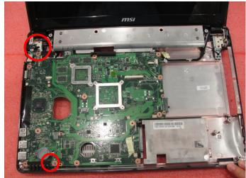
7.2 : Remove the 2screws (M2.5\*4mm).then remove the main board.
