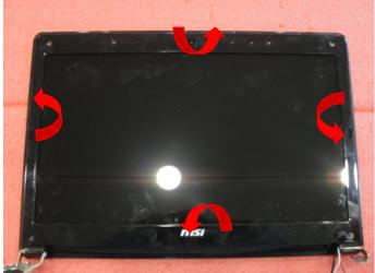
9.2: When removing the LCD bezel, should begin from the upside, then the two sides to downside.
