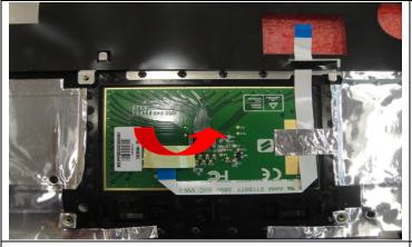
8.1: Release the connector that stabilize the T/P Cable, then remove the T/P module.
