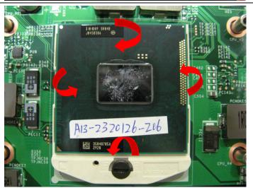
4.3: Open the CPU Slot with Screw Driver, then remove CPU Module as below.
