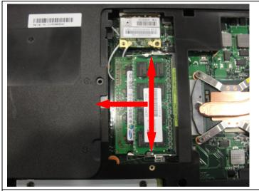
4.4: Push the two side shielding of RAM as pic shows; Then remove the RAM module according the direction as pic shows.
