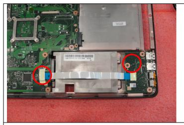
7.1 : Remove the 3screws (M2.5\*4mm).then remove the IO board.
