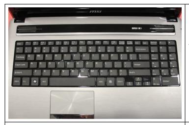
6.1: Remove the Keyboard. firstly from upside, then left side to right side, last remove down side.
