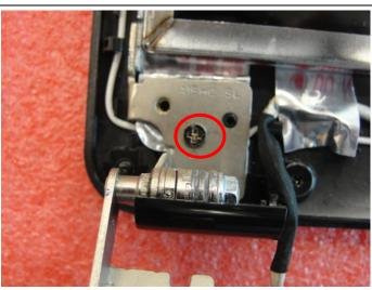
9.3: Remove the 1 screw (M2.5\*4mm), then remove the left hinge cap.
